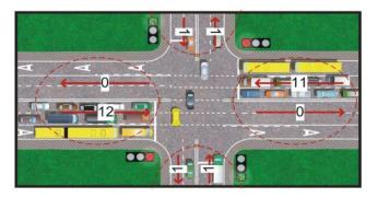
The Sensor can count the quantity of transport passing through the crossroads in two directions separately – to the Sensor and from it. Then these data can be transferred to control systems of the following crossroads to optimize the traffic lights operation and reduce a jam probability
