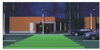
Pedestrian crossing control by occupancy - automatic lighting power change, control command transmission to traffic lights.
