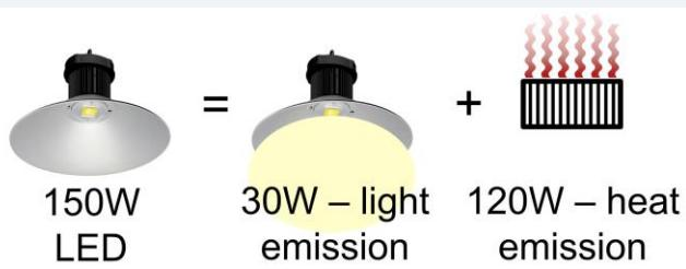
If food is stored in the warehouse, that is, the warehouse is artificially cooled, then it is necessary to consider the following. Nowadays, even the best LEDs use only 20 % of the energy for light emission and 80 % for heat generation. Therefore, the 150 W fixture is not only a light source but also a constantly working 120 W heater ( $150 \text{ W} \times 0.8 = 120 \text{ W}$ )!
